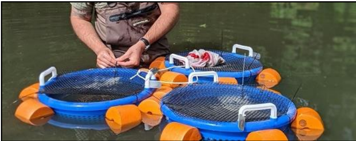
Figure 1. Three floating baskets, complete with can-floats and mesh lids, loosely connected with a tether.
