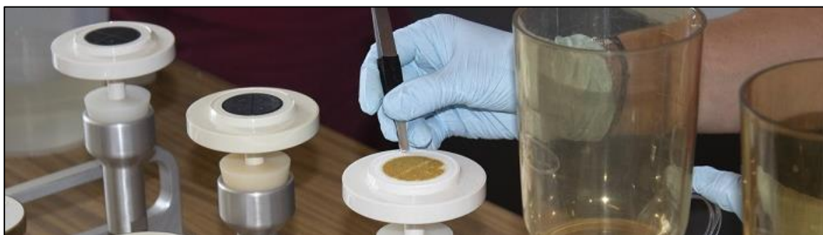
Figure 9. A technician collects a water seston sample using a filtration setup.
